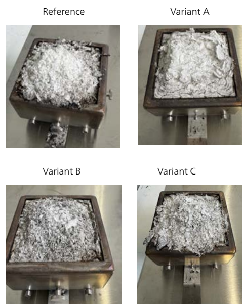
6 PVC samples after the measurement in the TCC 918
