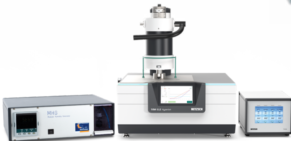
Humidity generator connected to the TMA 512 Hyperion ®
