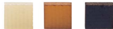
Typical de-coloration as a sign of beginning degradation: left: before measurement, middle: after being measured at 260°C, right: after being measured at 300°C. Neither of the measured specimens shows any visible delamination, although the TMA method is sensitive enough to detect it at 300°C.
