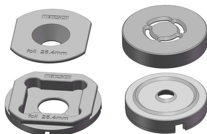
1 Sample holder for through-plane (left) and in-plane measurements (right) on thin foils
