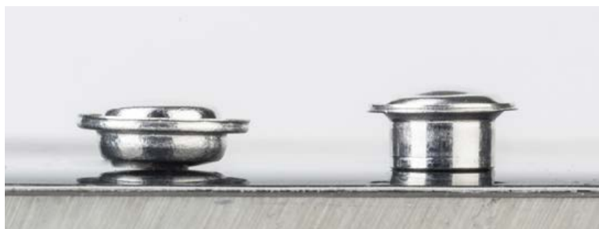
Fig. 3. Comparison of the two crucible types after heating to 600°C
