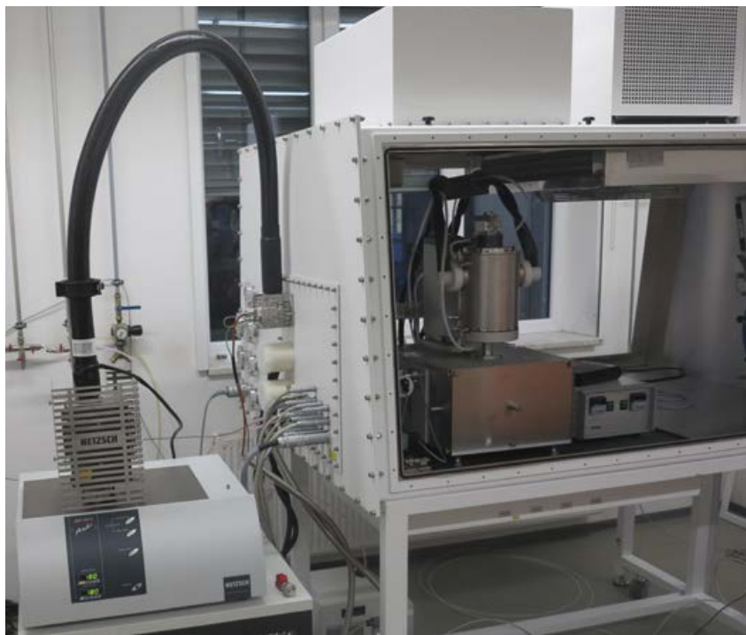
Fig. 1. STA 449 F1 Jupiter® glovebox design with heated feedthrough for coupling of the QMS 403 Aeolos®
