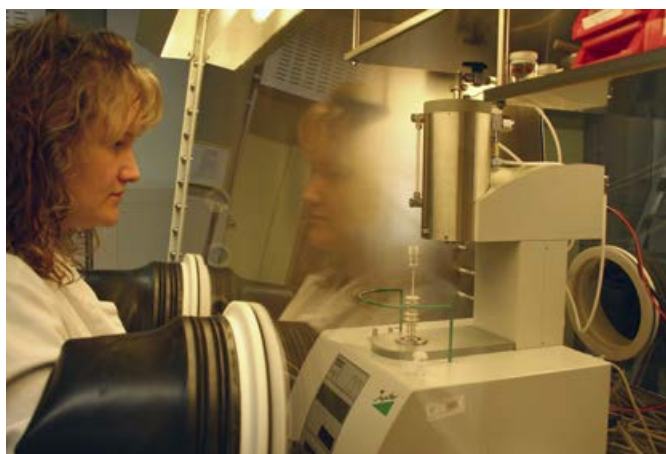
Fig. 6. STA 449 C Jupiter® in a material-protection glovebox at the Max-Planck-Institut CPFS Dresden (photo from "Picturebook 5", © M. Braun Inertgas-Systeme GmbH, Garching, Germany)
