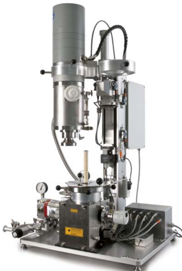
Fig. 5. Measuring part of the LFA 427 glovebox version
