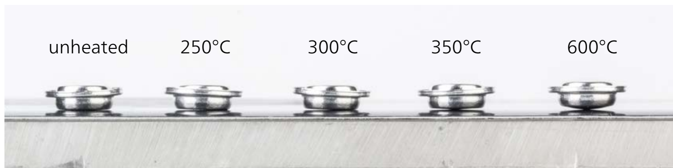
Fig. 1. Hermetically sealed standard aluminum crucibles at different temperatures
