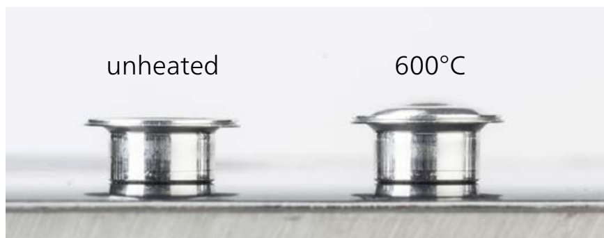
Fig. 2. Hermetically sealed Concavus ® crucibles at RT and 600°C
